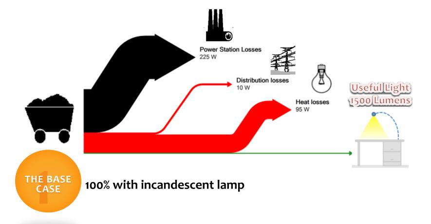
Energy service delivered is a fraction of the fuel fed into a power plant
