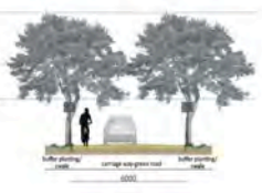
A.4 SECTION THROUGH 6 M WIDE ROAD
