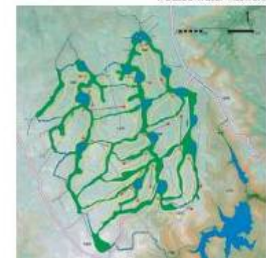
Figure 6 : Grey water and sewage network
