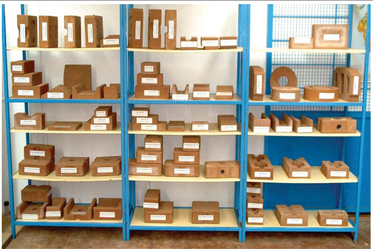
Compressed Stabilised Earth Blocks (CSEB) by the Auram press 3000 17 moulds for doing about 75 different blocks
