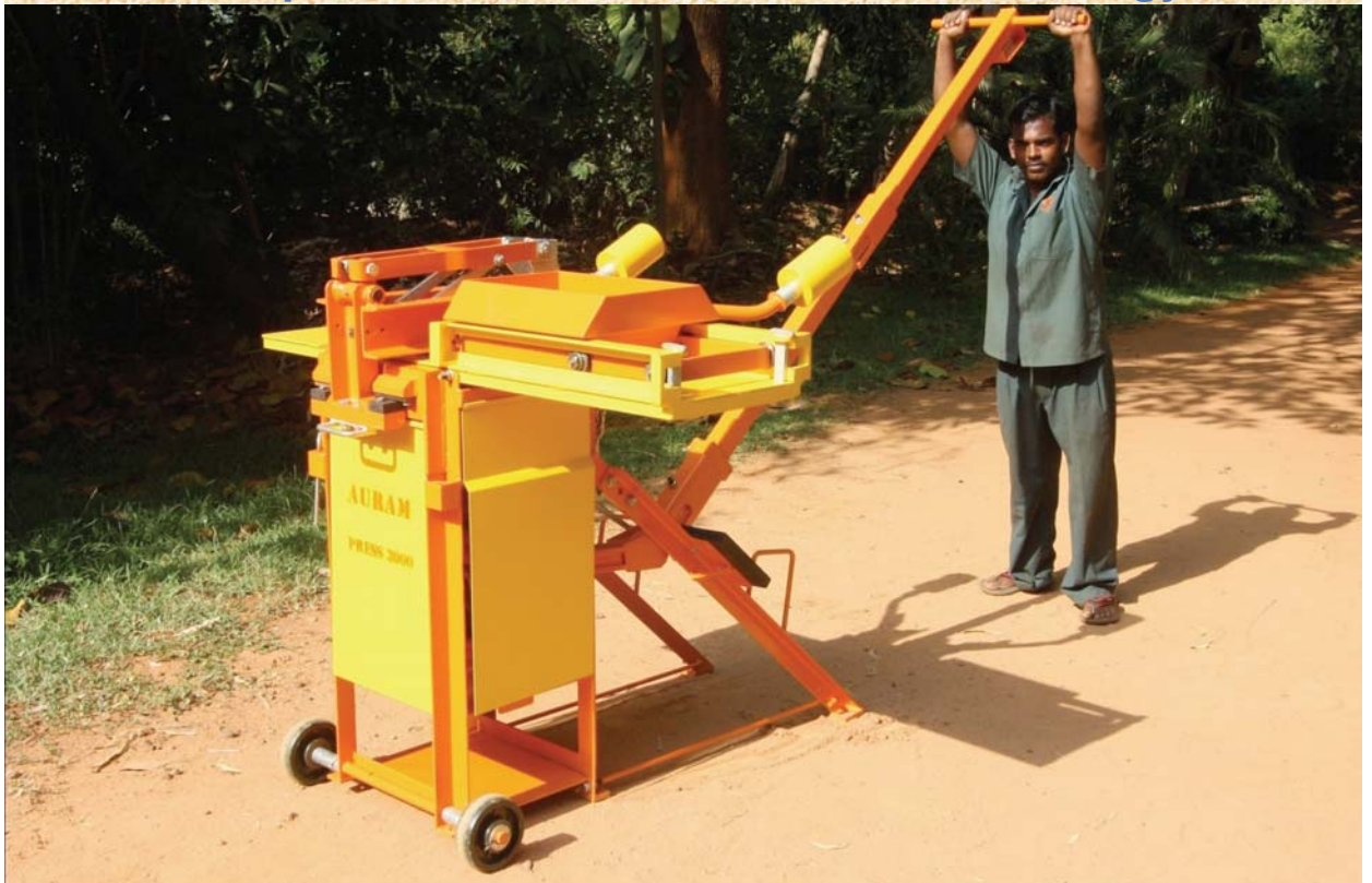
Auram press 3000 - Multi mould manual press with 17 moulds for doing ~ 75 blocks
