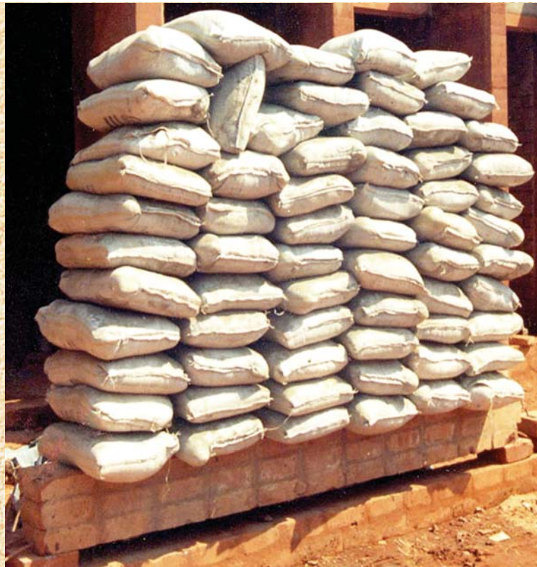
Testing a triple height composite beam 240 2.50 m span, 1280 Kg/m, 4 mm deflection, no cracks
